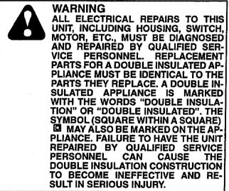
This unit is Double Insulated to help protect against electric shock. Double insulation construction consists of two separate "layers" of electrical insulation instead of grounding.
